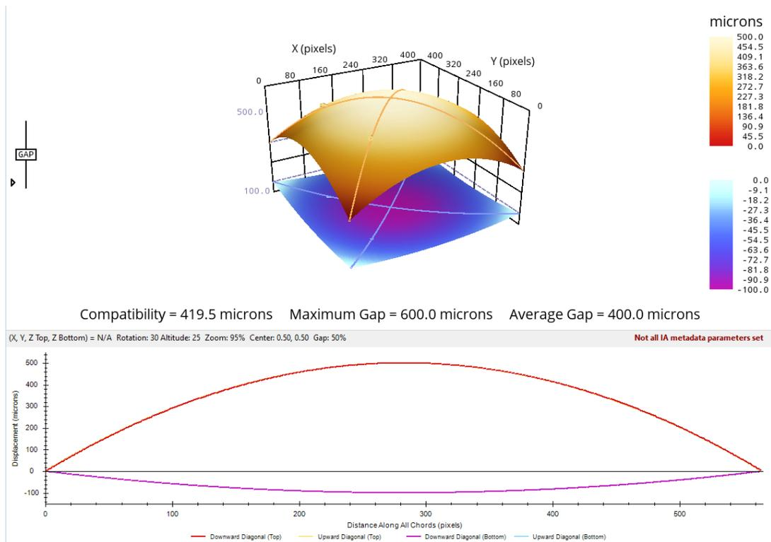
Figure 9. Interface Analysis of Poorly Matched Mating Surfaces
