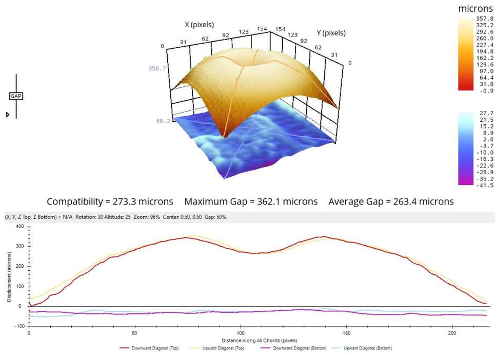
**Figure 12. Solder Liquidus (220°C) Interface Analysis between Smaller BGA 1 and PCB 1 – ROI 2**
