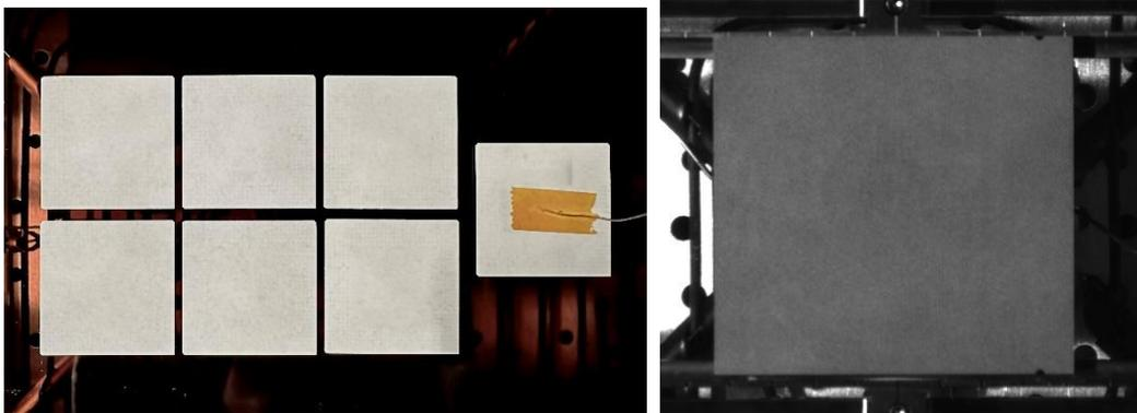
**Figure 6. Package Samples (Smaller BGAs: left, Larger BGAs: right) Test Setup in Oven**
