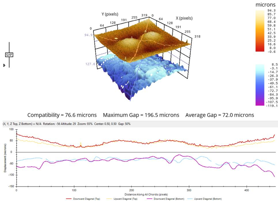
**Figure 11. Room Temperature Interface Analysis between Larger BGA 4 and PCB 1 – ROI 2**
