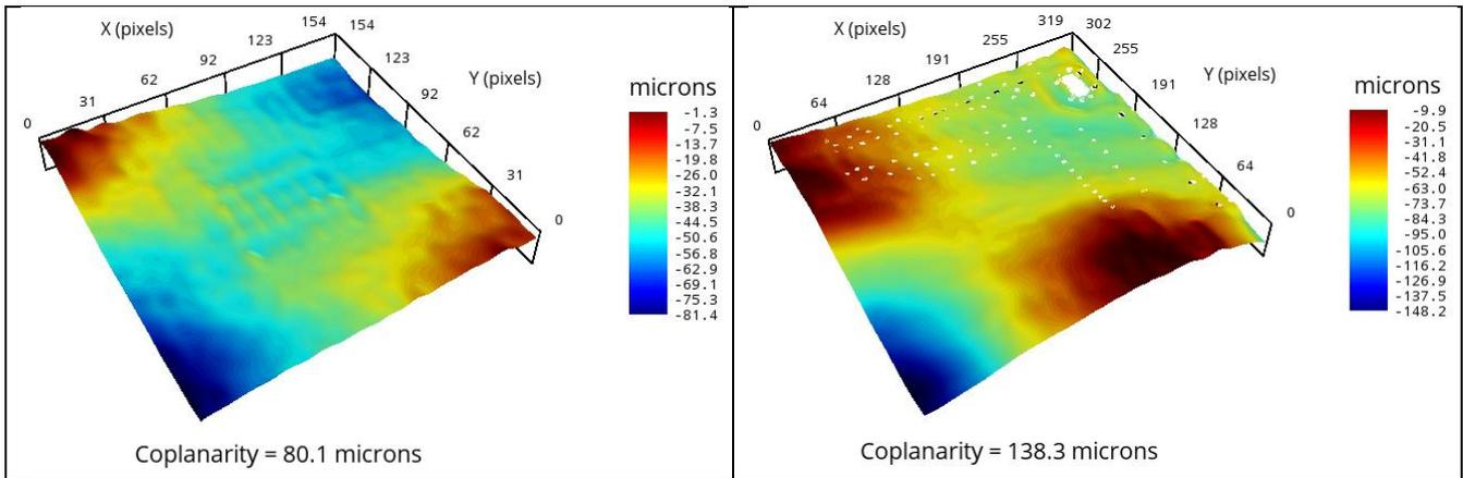
**Figure 15. Average Relative Shape Change from Room Temperature to 220°C; Smaller BGA (top left), Larger BGA (top right), Smaller PCB all ROI (bottom left), Larger PCB all ROI (bottom right)**
