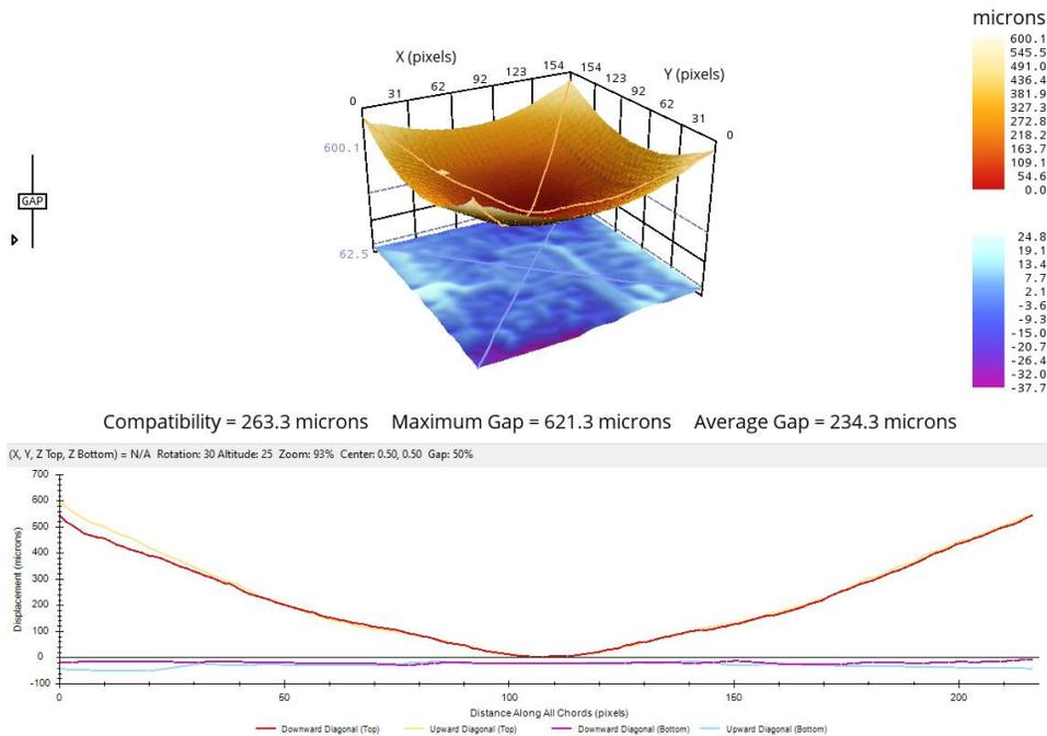
**Figure 10. Room Temperature Interface Analysis between Smaller BGA 1 and PCB 1 – ROI 2**
