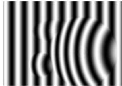
Figure 4. Digital Fringe Projection Pattern
