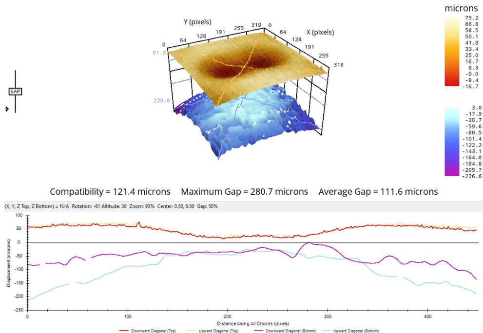
**Figure 13. Solder Liquidus (220°C) Interface Analysis between Larger BGA 4 and PCB 1 – ROI 2**
