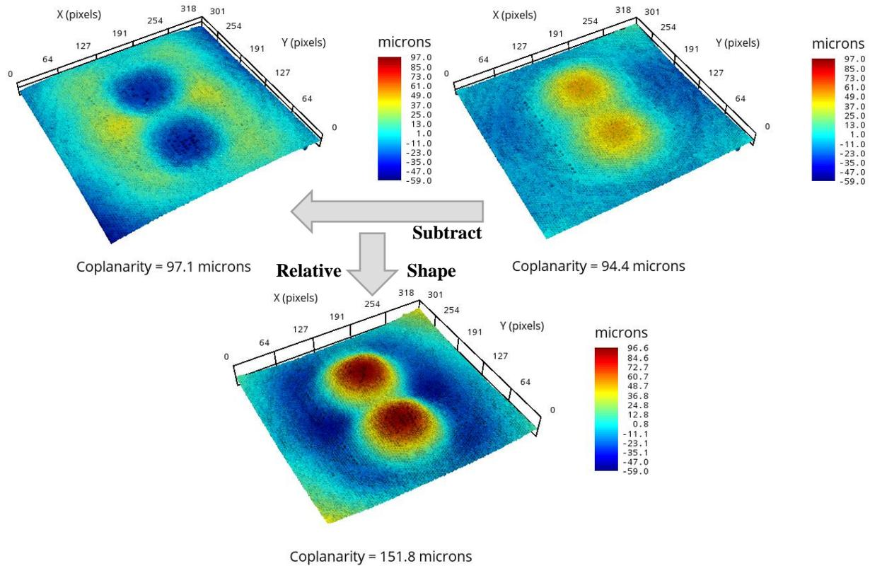
**Figure 14. Relative Shape Change in BGA 4 from Room Temperature to 220°C**
