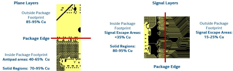
90 91 Figure 4 Representative Retained Copper Outside & Inside a Package Footprint Area 92
