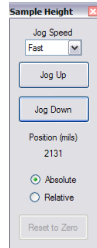
Figure 2.2 Sample Height Adjust Window
