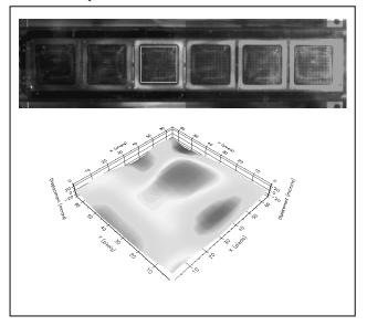
Post-processing test and inspection revealed that defects existed in roughly 5% of the lot. Additional analysis of the pre-production coplanarity data yielded a strong correlation between the 5% fallout and coplanarity values (relative) between -3.0 mils (-51 µm) and -1.7 mils (-43 µm). Approximately 80% of the interconnect (die – flex) defects had pre-production coplanarity values between -3.0 mils (-51 µm) and -1.7 mils (-43 µm).
