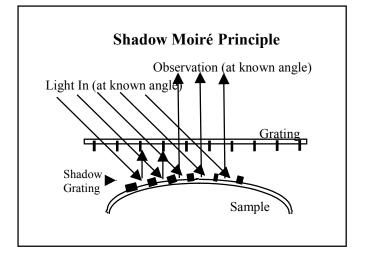
When the surface of the sample deviates from a flat plane or is not parallel to the grating, fringes are visible. In the event that a sample is perfectly flat and positioned parallel to the reference grating, no fringes are present. From the governing equation of shadow moiré,
