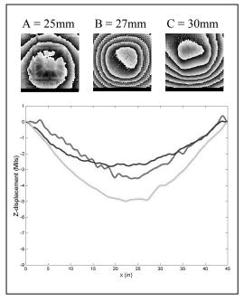
**Figure 6.** Innermost row of solder ball pads are analyzed for maximum deflection.
