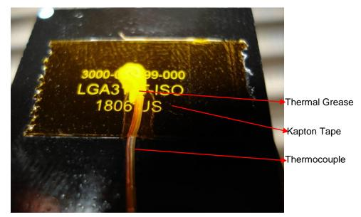
Figure 3 Thermocouple Placement
