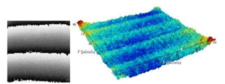
Figure 1 Phase Image with resulting 3D Surface showing periodic ripples
