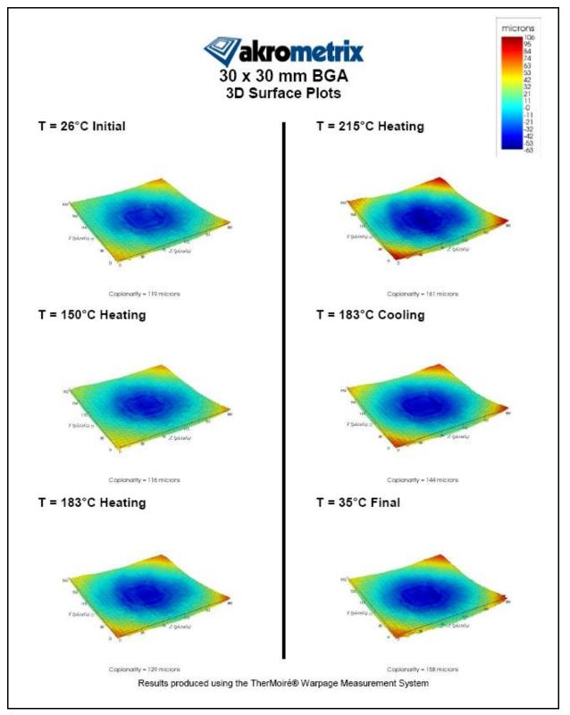
Figure 5 Akrometrix Component Report with 3D Surface Plots
