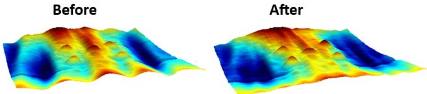
In Shadow Moiré measurements, a primary fringe pattern is generated by the interference between the grating lines and the shadows they cast on a sample surface. Certain repetitive features on the surface can produce an additional, secondary interference pattern. This can sometimes be mitigated by rotating the sample relative to the grating lines or by painting the surface.
