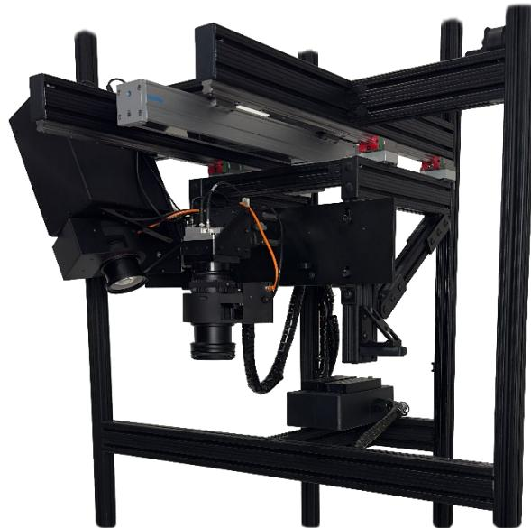
Automation includes moving the camera and projector assembly in and out of the oven using **NAVIGATE TO LOAD OPTION**. This capability makes switching between Shadow Moiré and DFP measurements much easier, as the adjustable assembly allows users to transition smoothly between the two techniques.
