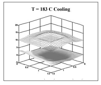
In this example a pre-production evaluation/qualification of temperature dependent behaviors could have alerted the assembler of the likelihood of defects due to the magnitude of warpage experienced during thermal loading.
