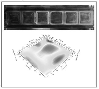
Post-processing test and inspection revealed that defects existed in roughly 5% of the lot. Additional analysis of the pre-production coplanarity data yielded a strong correlation between the 5% fallout and coplanarity values (relative) between -3.0 mils (-51  $\mu$ m) and -1.7 mils (-43  $\mu$ m). Approximately 80% of the interconnect (die – flex) defects had pre-production coplanarity values between -3.0 mils (-51  $\mu$ m) and -1.7 mils (-43  $\mu$ m).
