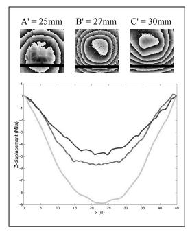
Figure 7 shows the flex-BGA substrate (typical) and its resulting 3D surface plot from shadow moiré data. Coplanarity is given for the die attach area (22 mm X 22 mm inspection area). In this evaluation, an approximate 12% of die attach areas failed the 3.0 mil coplanarity limit.
