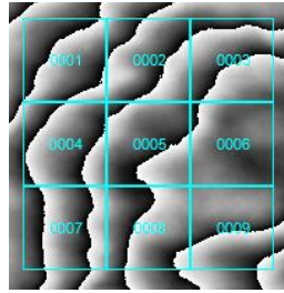
Figure 3.31 Example of a Partition Array
