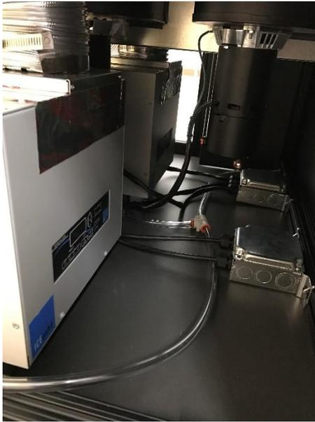
**Figure B.2** Drain Hose Routing
