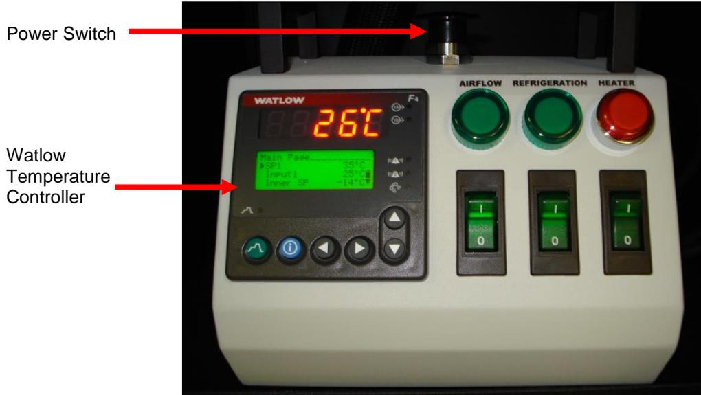
**Figure 1.6** Temperature Controller Front Panel Controls
