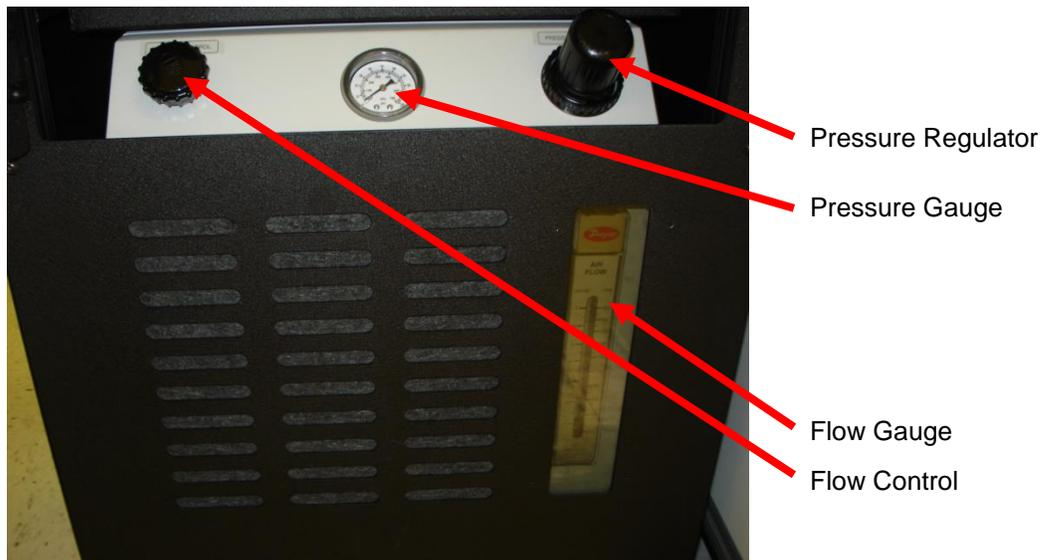
Figure 1.4 Air Chiller Front Panel Controls
