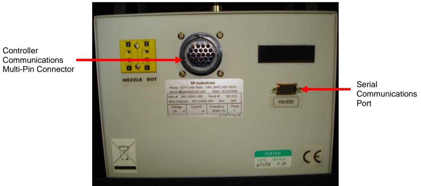
Figure 1.7 Temperature Controller Back Panel Connections
