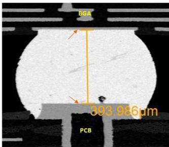
Figure 2. Standoff measurement
