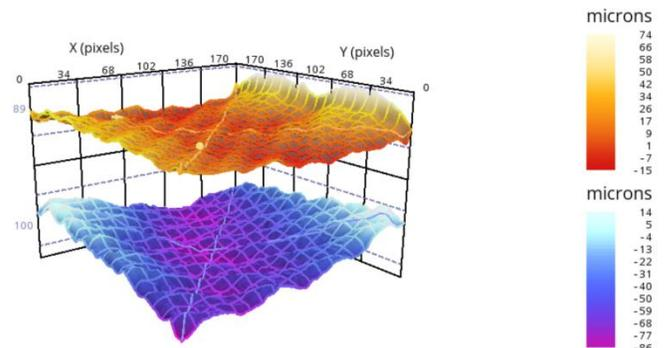
Figure 6. Interface Analysis Example, BGA to PCB
