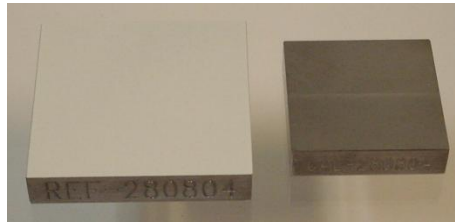
Figure 3.4 Reference Plane and Calibration Blocks
