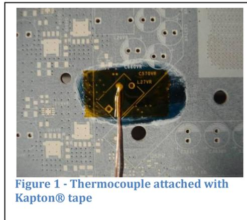
Figure 1 - Thermocouple attached with Kapton® tape
