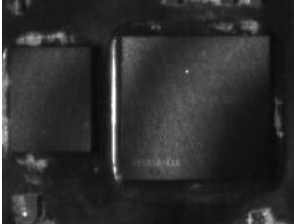
Figure 4. Exposed die shadow moiré image
