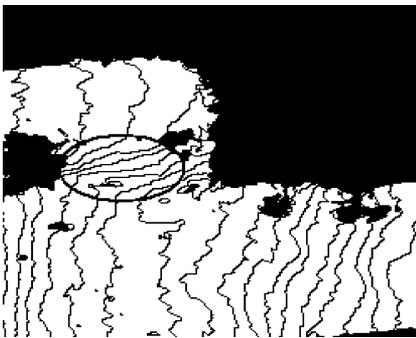
Fig. 13. Close-up of computer enhanced moiré fringe contours of horizontal displacement on outside bump (circled) of 16 I/O MicroCSP. Contour interval is 100.4 nm.
