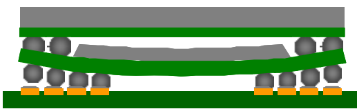
Figure 7: Mechanism of open joints
