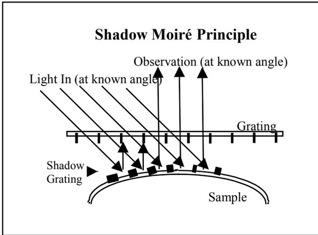
When the surface of the sample deviates from a flat plane or is not parallel to the grating, fringes are visible. In the event that a sample is perfectly flat and positioned parallel to the reference grating, no fringes are present. From the governing equation of shadow moiré,
